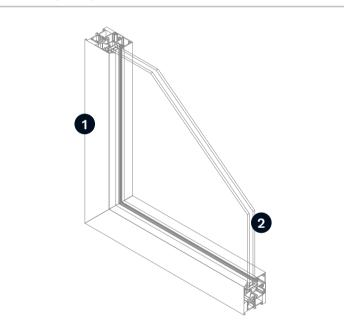
Aluminium profile carpentry with thermal bridge break
