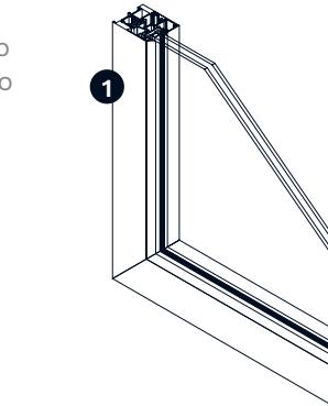
① Aluminum profile with thermal break
